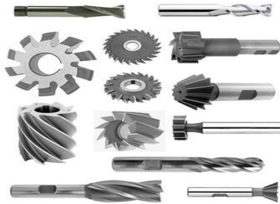
Fig.4 Multipoint cutting tools
