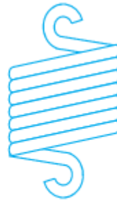
(b) Tension helical spring.
