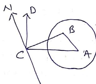
The sides of the  $\triangle ABC$  must be measured very carefully with a tested steel tape. When the angle at A & C are very small, the sum of the length of the two short sides of the triangles is virtually equal to the length of the longest sides, the difference being so small as to be scarcely, almost not measurable.
