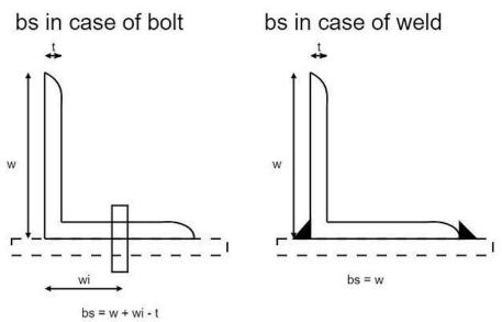
But for preliminary sizing, the rupture strength of net section may be approximately taken as
