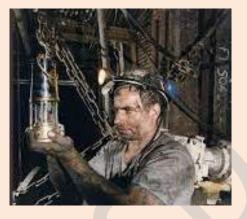
3. No efforts should be made to raise the flame safety lamp higher than is necessary to test for accumulation because this results in keeping the flame in richer mixture of methane and air which may explode inside the lamp and extinguish the flame.
