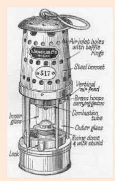
(h) Outer & Inner gauze : To prevent the passage of flame from interior of lamp and the heat absorbed purpose.
