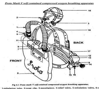
1-exhalation tube, 2-nose clip, 3-mouthpiece, 4-relief valve, 5-exhalation valve, 6-cooler, 7inhalation valve, 8-pressure gauge valve, 9-breathing bag with inhaling and exhaling compartments, 10-head harness, 11-pressure gauge, 12-pressure gauge tube, 13-oxygen supply tube, 14-cylinder valve, 15-press button bypass valve, 16-reducing valve, 17-oxygen cylinder, 18-inhalation tube.
