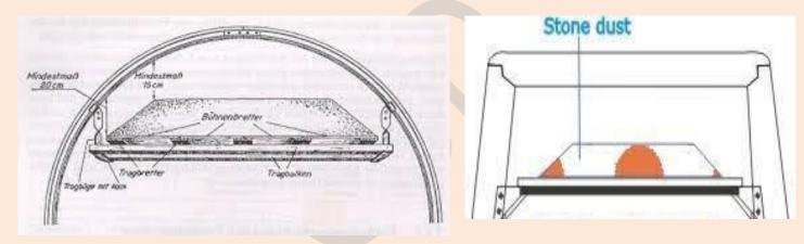
In this type of barrier the stone dust rests on planks which run longitudinally in the road way and whose length equals the width of the shelves. These planks rest on a rigid frame, the two main members of which are at least 150 mm in depth and rest on their edges on two fixed rigid brackets. Neither the frame, nor the planks are fastened either to each other or to the fixed brackets.
