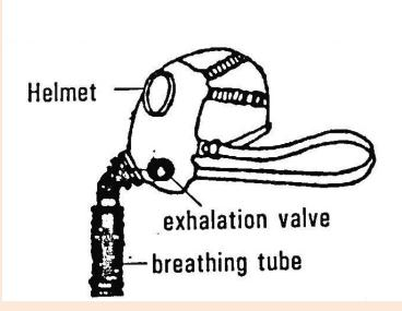
The helmet totally covers the face and head of the wearer and is provided with a flexible hose pipe of 25 mm bore, 30 m long.
