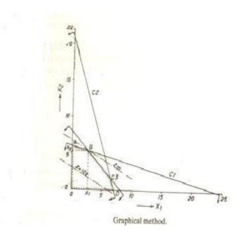
Mark the point of 24 at X1 axis and point 6 on x2 axis. The straight line represents c1 equation.
