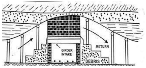
According to Indian regulations, air crossing should be fireproof and in gassy coal mines, explosion proof too. They should be of a minimum thickness of 250mm if constructed of brick or lightly reinforced concrete or of 150mm if constructed of properly reinforced concrete. Sometimes brick or concrete arches may be used instead of the rectangular construction.
