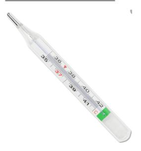
A Medical thermometer is used to measure body temperature. Most thermometers made in the 20th century are mercury thermometers. They are sensitive and accurate, having a narrow place where the level of mercury rises very fast. A kink on the tube stops the mercury level from falling on its own.
